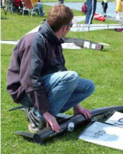
**'Tube Too'** demonstrated the reaching and marginal planing ability of an even narrower, totally circular sectioned hull with a maximum diameter of 118mm, a displacement of 4.8kg and a draught of 617mm"
